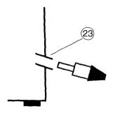
The temp. control unit is drained at the nozzle 23.
