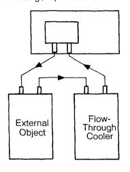
With immersion and flow-through coolers from HAAKE, the heat transfer liquid can be cooled down considerably below 0°C and the circulator can be rendered independent of tap water.
